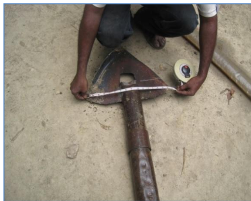
Figure 8: The 46 cm drill bit
