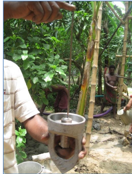
Figure 13. The plug fitted to close the hole of the plug cutter
