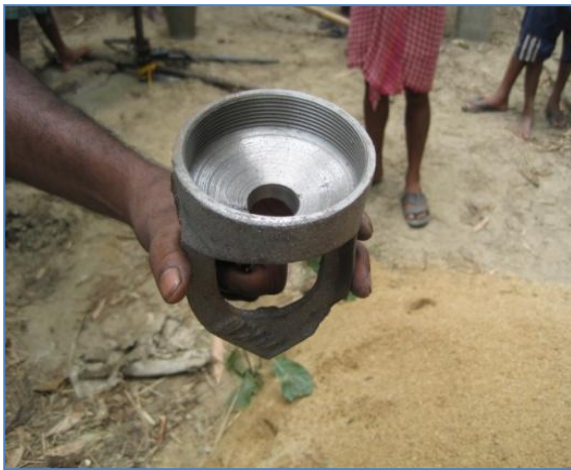
Figure 12: The plug cutter
